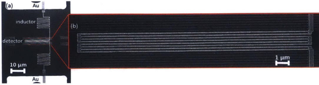
Figure 3-9: SEM of waveguide-detector. (a) The detector is shown with the series inductor consisting of 300-nm-wide nanowires. (b) Magnified SEM of detector region encircled with red lines in (a). The detector consists of four 2-SNAPs in series with each 2-SNAP comprising two \sim 60 - to 80-nm-wide nanowires in parallel.
