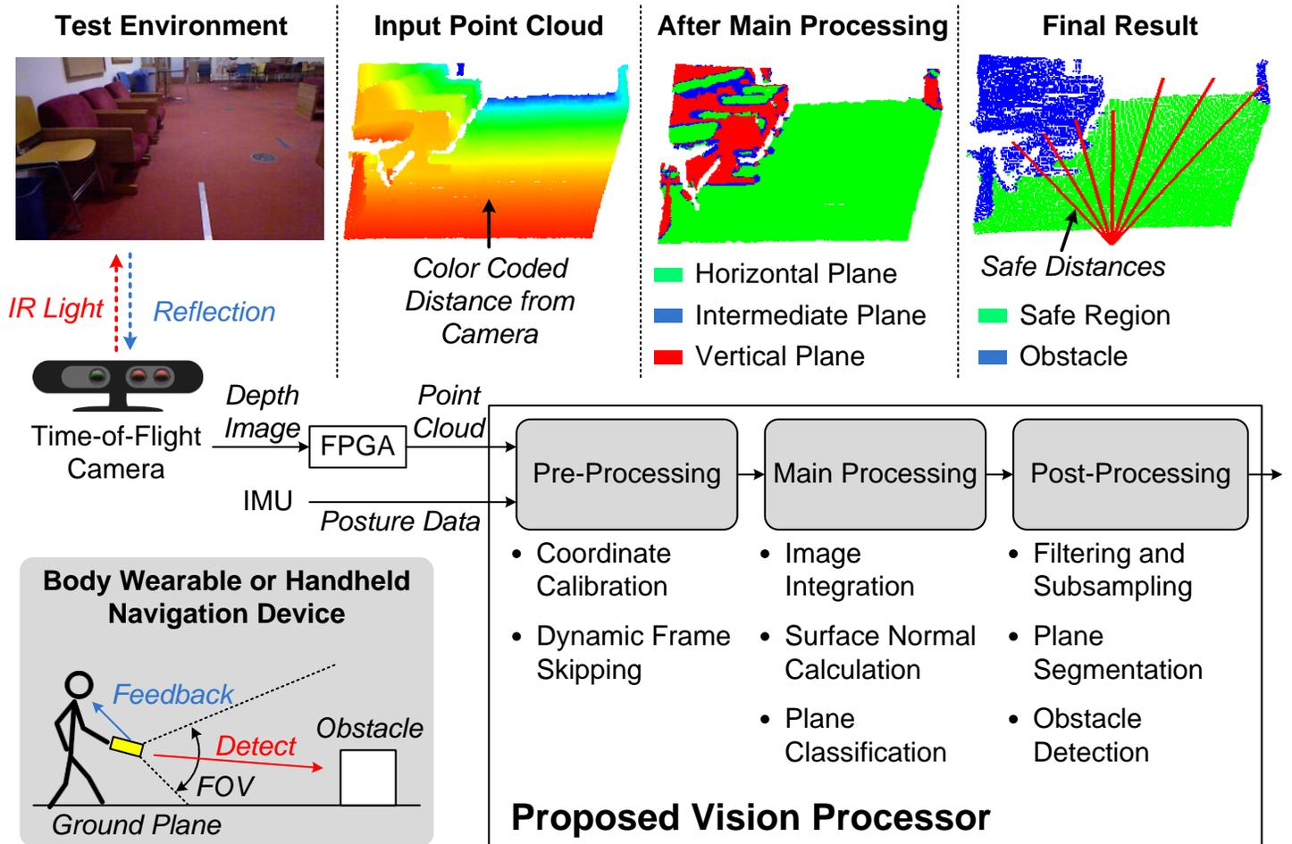
Figure 1. Overview of a navigation device for the visually impaired. The device is designed as a body wearable or handheld system which can replace a conventional cane.
