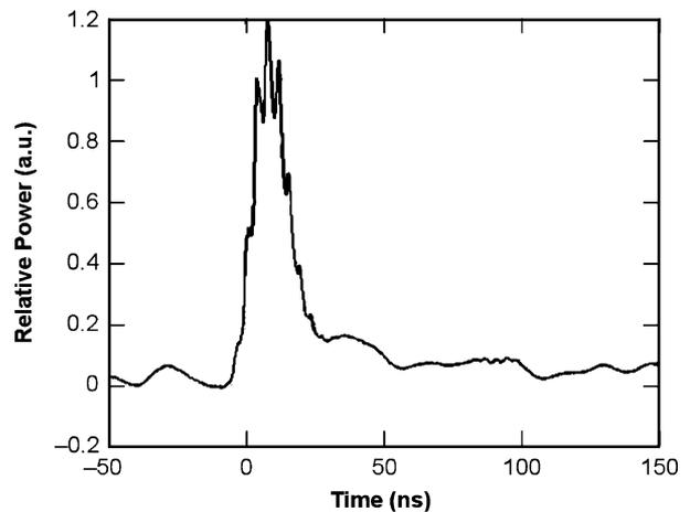
Fig. 3.  $Q$ -switched pulse shape (114 W, 5-kHz PRF). The FWHM of the pulse determined by a polynomial fit is 16 ns. The structure in the pulse is due to longitudinal mode beating that is only partially resolved by the scope (500 MHz bandwidth).
