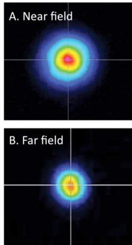
Fig. 4. (A) 1:1 image of the beam at the output coupler (Q-switched, 114 W). Beam diameter is 1.2 mm ( $1/e^2$ ). (B) Far-field beam profile at focus of 25-cm FL lens. Beam diameter ( $1/e^2$ ) at focus is 260  $\mu\text{m}$  at 114-W output power.
