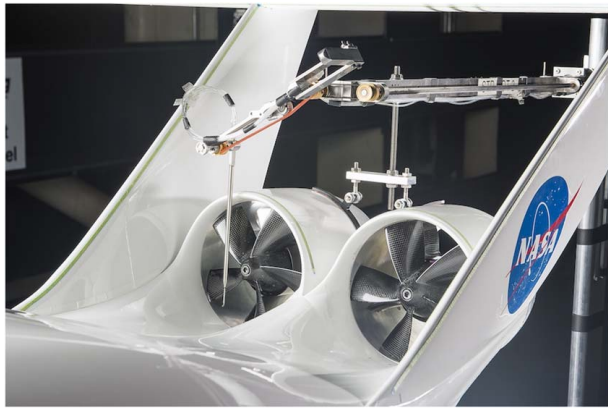
Fig. 2 Boundary layer ingesting ducted fans integrated into D8 wind tunnel model empennage with five-hole probe inlet traverse system (photo credit: NASA/George Homich)
