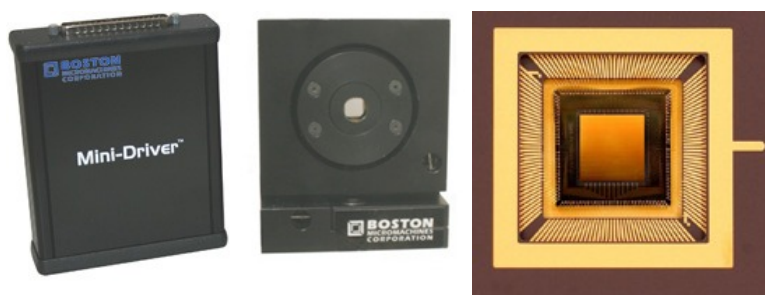
Figure 1: Boston Micromachines Mini 6 \times 6 (32 actuator) deformable mirror and drive electronics [39]. The drive electronics board would be used without the packaging and with some minor modifications to the board.
