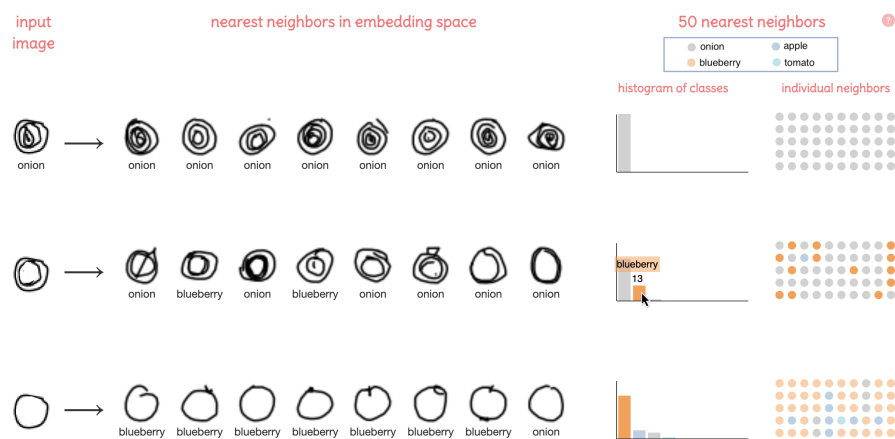
Figure 5-10: An interactive prototype of the NN interface for the Quick, Draw! dataset juxtaposes neighbors side-by-side instead of overlaying them. Input editor operations include drawing, erasing or adding shapes. In this figure, for example, we show how using an “erase” tool to remove inner rings from the input image (an onion) changes the neighbors to almost all blueberries instead, suggesting that the model has learned a correlation between inner circles and the onion class.
