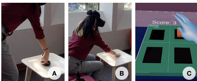
Figure 3: The user aligns the controller against a table surface to place the game platform (A). They can tap on the table and receive haptic feedback (B) as they hit the virtual moles in the Whack-a-Mole game (C).
