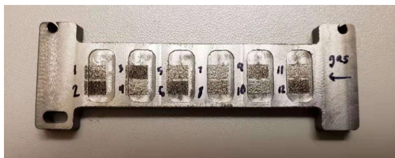
Figure 33: Nb substrate with single-layer prints of Nb powder in machined wells
