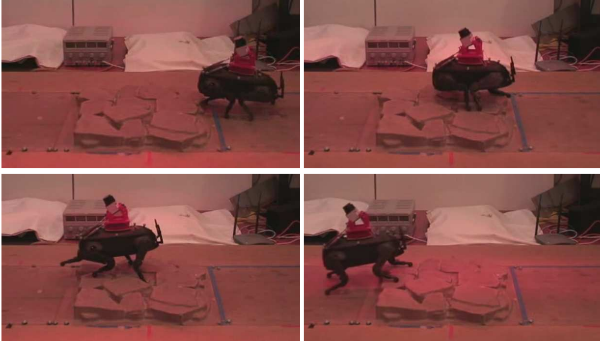
Figure 17: Snapshots of a video documenting the walk over the terrain using the learned terrain model from own elevation observations (from top left to bottom right).
