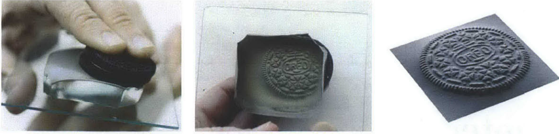
Figure 2-1: An example of the coated elastomer displaying the surface pattern of a cookie, and the reconstructed cookie surface.[18]
