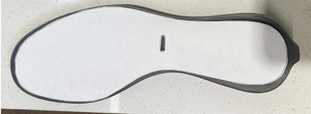
Figure 16: Paper template used to mark bending location on test samples
