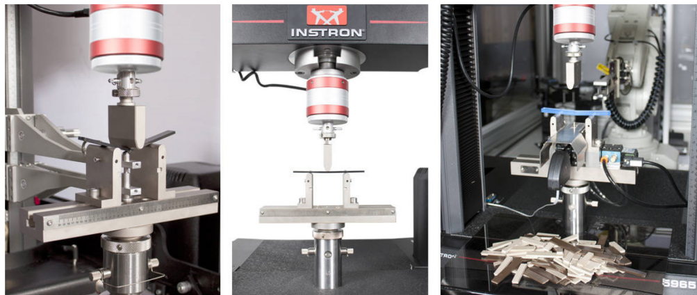
Figure 9: Example of a three-point bend test set-up on a universal testing machine [20]
