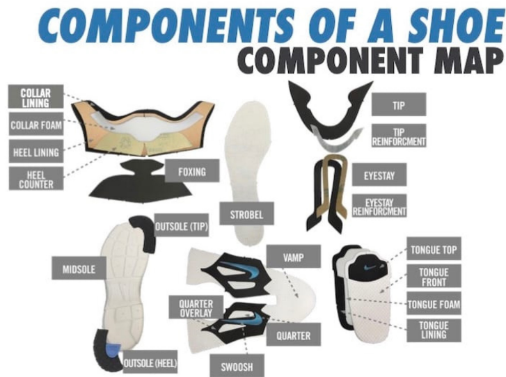
Figure 4: Breakdown of separate shoe components for an athletic shoe [4]
