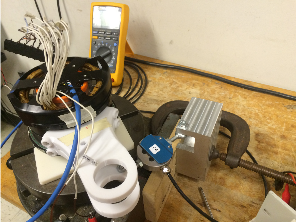
Figure 8-5: Photo of test setup, showing motor mounted in housing. Housing is mounted to milling turntable, and output arm is connected to load cell. The phases are connected together with the terminal block shown at the upper-left of the photo.
