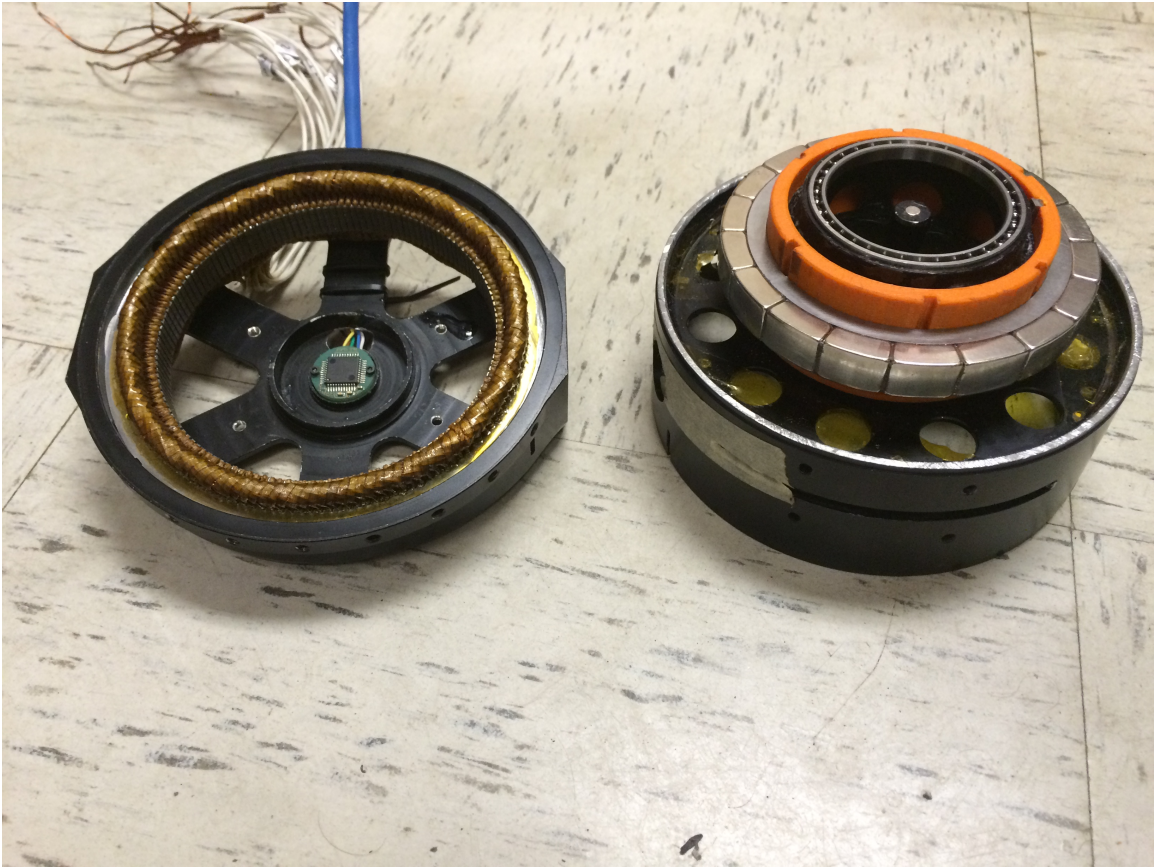
Figure 8-1: Stator (left) and permanent-magnet rotor (right). Circuit board is magnetic encoder. Orange cylinder is the 3-D printed spacer with keyways. Shaft encoder is visible in the center of both rotor (magnet on post) and stator (integrated circuit).
