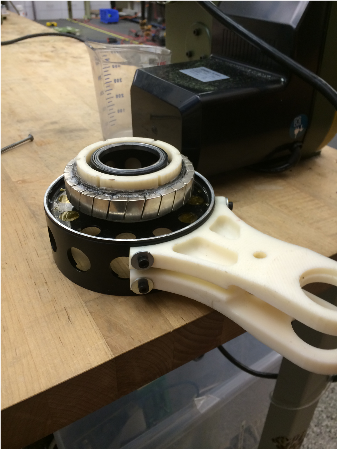
Figure 5-2: Skewed magnets in rotor
