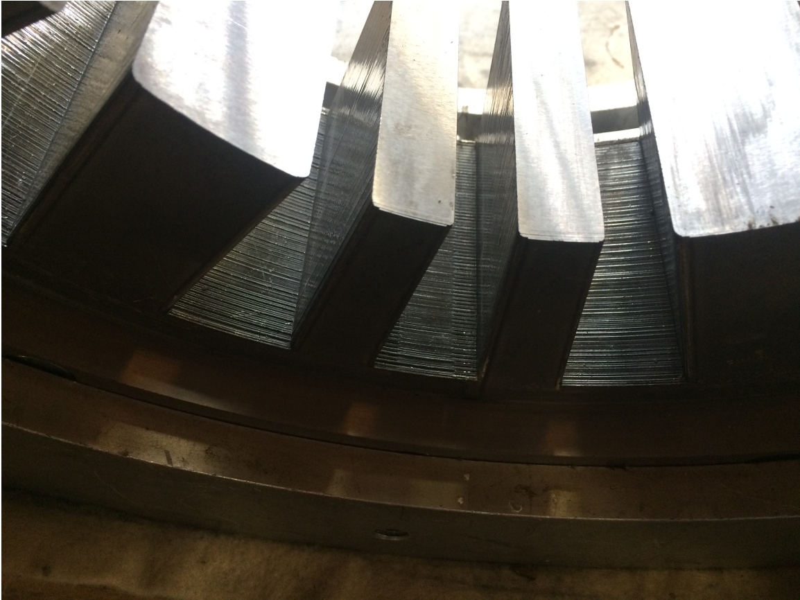
Figure 10-4: Chamfered edges on example electric machine stator
