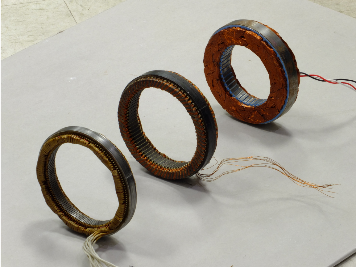
Figure 11-1: Comparison of Stators: 8-phase (front), 3-phase gen-2 (middle), 3-phase commercial solution (back). Each successive stator represents an increase in absolute torque production, a decrease in mass, and an increase in efficiency in the application in question.
