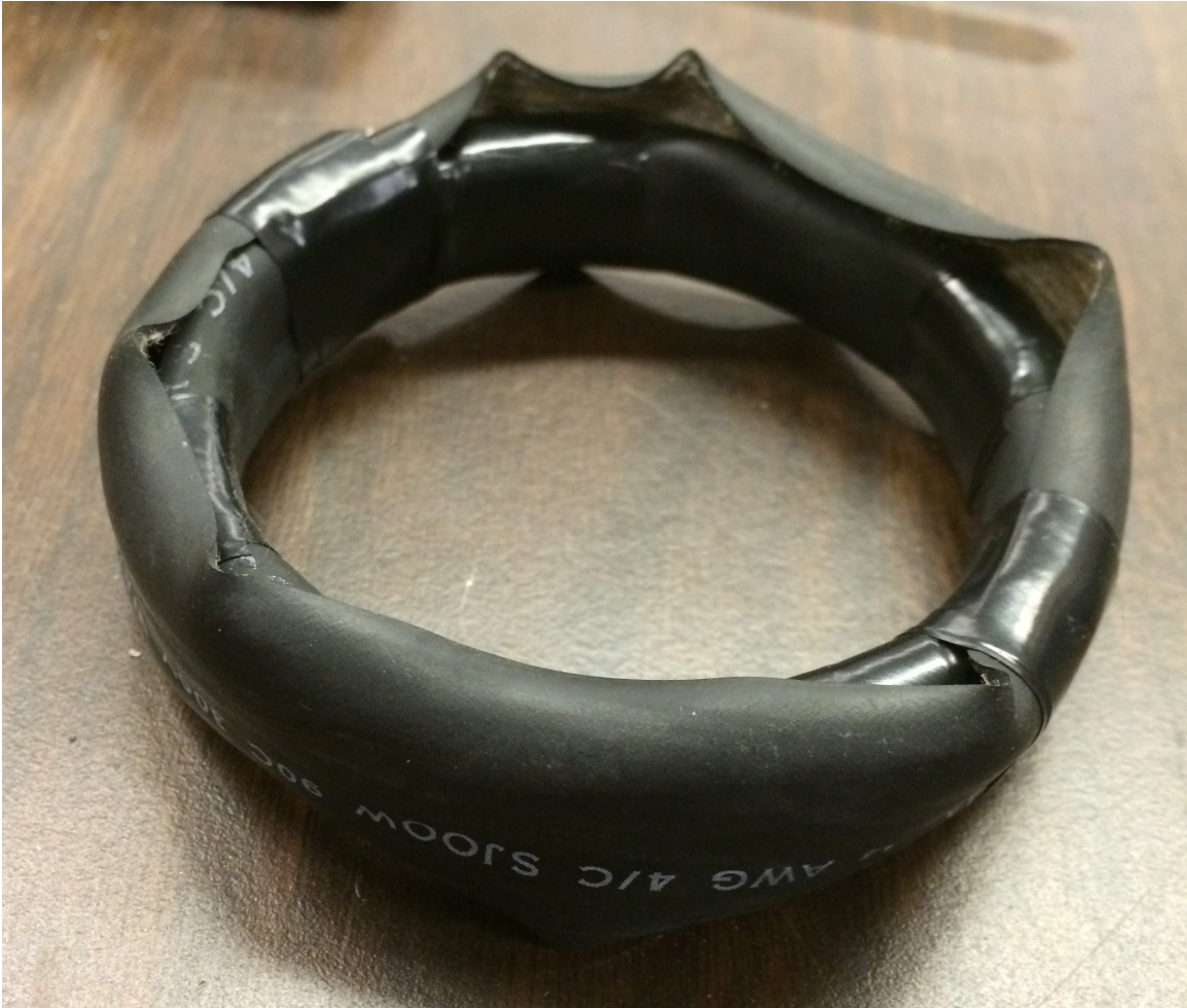
Figure 6-2: Rubber insulation taken from large 4-conductor cable
