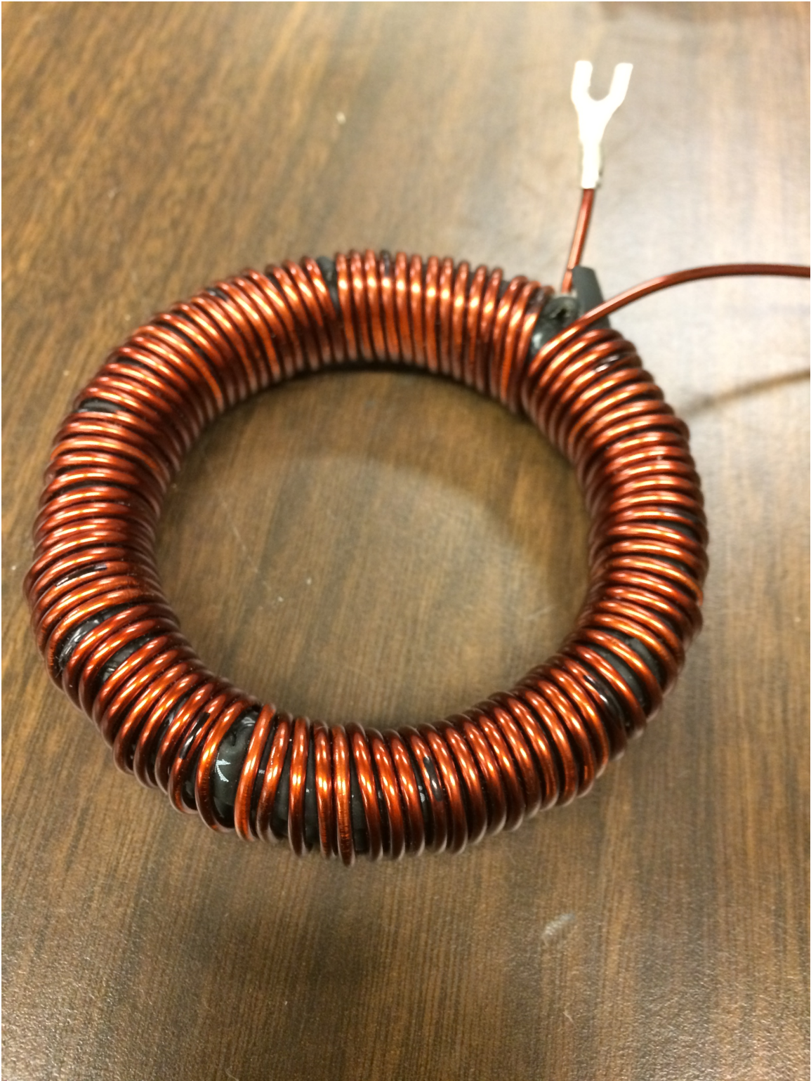
Figure 6-3: Wire wrapped around protected core
