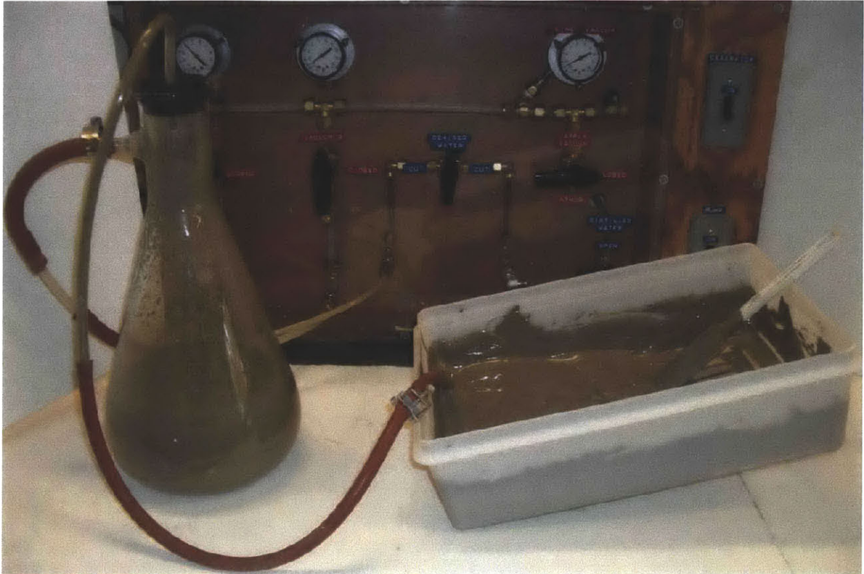
Figure 3-1: Vacuum setup used to de-air RBBC slurry
