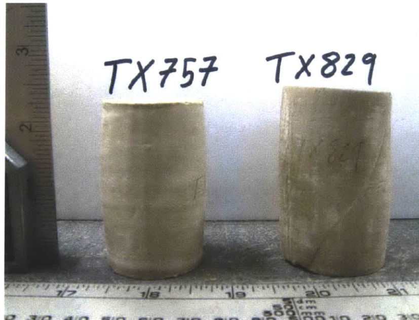
Figure 2-28: A picture of NC RBBC specimens after CK_0UC tests showing a bulging mode of failure for the low pressure test (TX757, \sigma'_{ac} = 0.67 MPa) and a slip surface for the high pressure test (TX829, \sigma'_{ac} = 9.74 MPa) (Abdulhadi, 2009)
