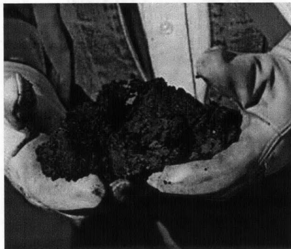
Figure 2-3: A photo of the oil sands (Source: Canadian Association of Petroleum Producers [CAPP])
