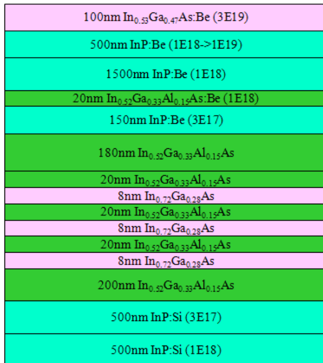
Figure C-5: The layer structure for VA159, one of the strained InGaAs quantum well laser structures investigated in Section 3.2 and Chapter 4.
