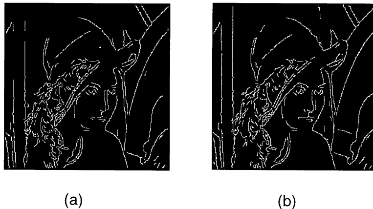
Figure 4-1: (a) Binary edge map with low Sobel threshold of “Lenna” at 0.275 bpp.(b) Binary edge map using hybrid method at 0.270 bpp.
