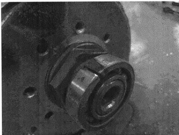
Figure 19: Removing the unsealed bearings Figure 20: magnetic dust on the rotor
