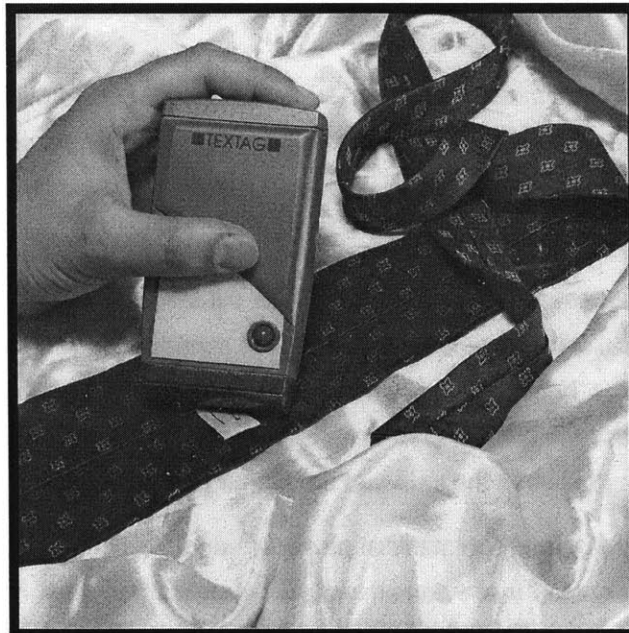
Figure 56. Photograph of a hand-held reader used for authenticating goods. This particular tag and reader do not provide any ID information and only indicate presence.
