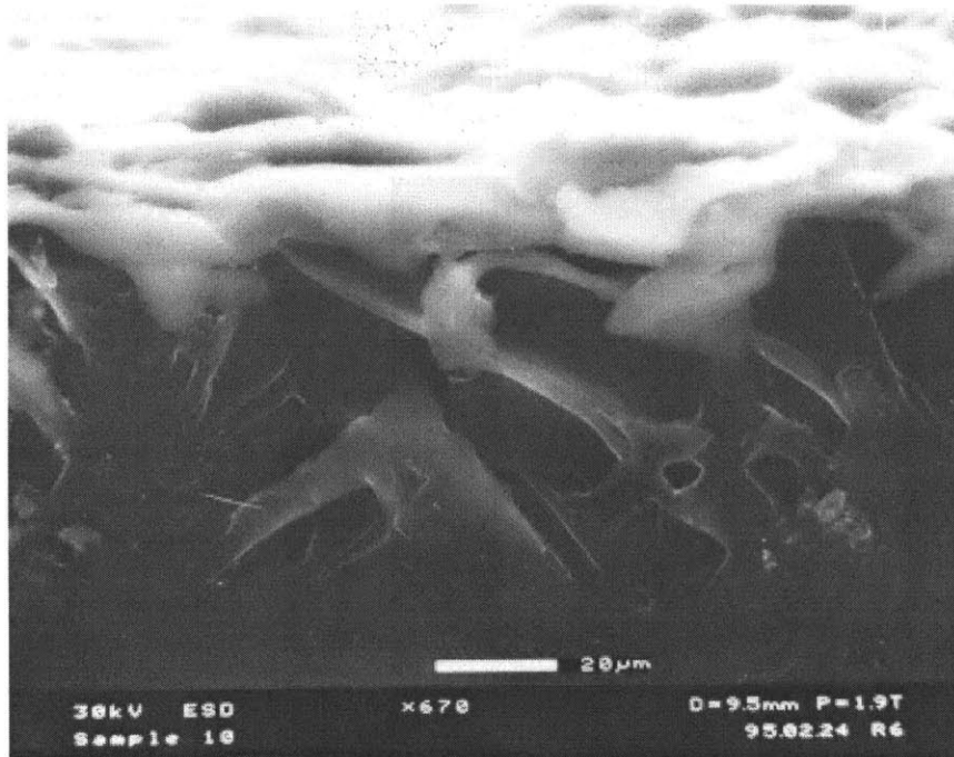
Figure 110. SEM cross section of a force sensor made by Interlink, Inc. showing a metallized layer over a bed of conductive elastomer cilia-like structures. As the material is compressed, the increased interconnection within the material structure increases the number of conduction paths and reduces the electrical resistance of the structure. On this microscopic scale, it is easy to see why the electrical resistance is not a smooth continuous function of the applied force.
