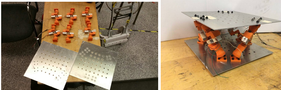
Figure 2-4: The small hex sensor's legs and platform before assembly, and the completed hex sensor.
