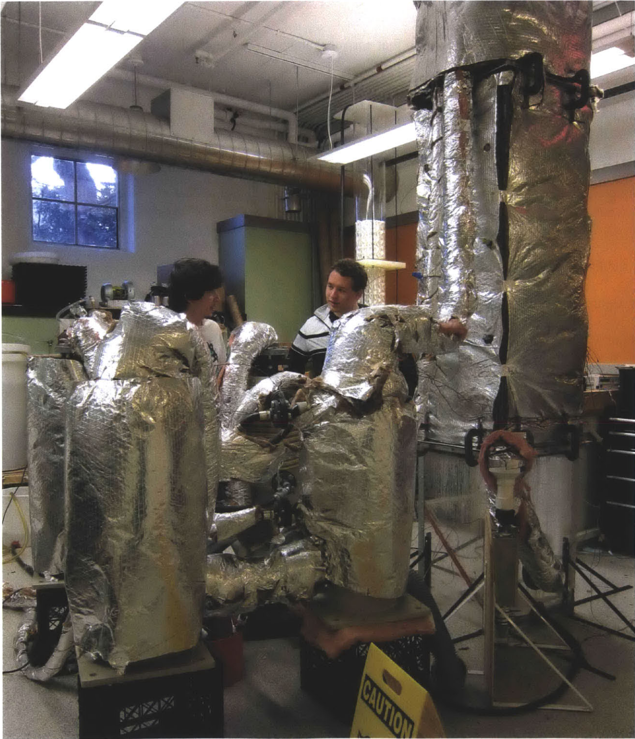
Figure 2-1: HDH Experimental Plant
