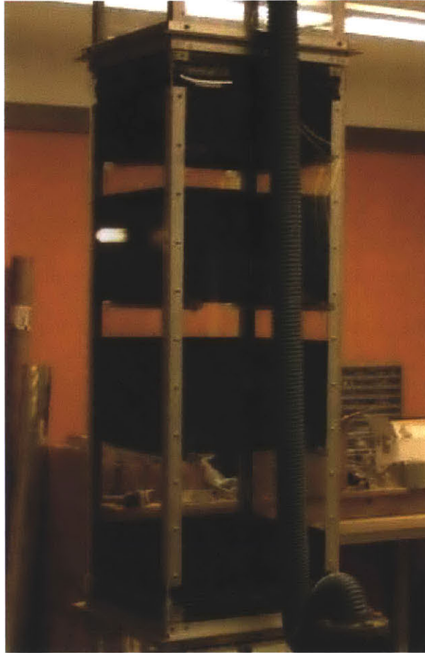
Figure 2-6: Heat Transfer Fills in the Middle Section
