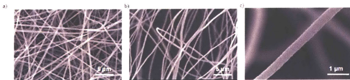
Figure 6-1. (a) SEM images indicate that electrospun PAN nanofiber mat consists of smooth and continuous fibers with diameters of 300-500 nm. (b) Carbonized electrospun fibers maintain their continuous fibrous structure. (c) The electrospun CNFs show surface roughness under high magnifications.
