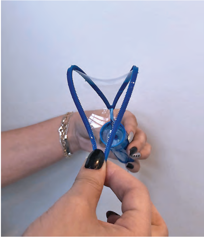
Figure 19. A soap film is a solution to the Dirichlet problem of finding a conformal harmonic map with prescribed boundary.
