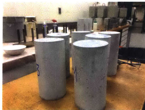
Figure 19: Cylinders collected from concrete batches
