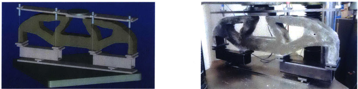
Figure 22: CAD model of beam in testing apparatus, and photo of beam in testing apparatus
