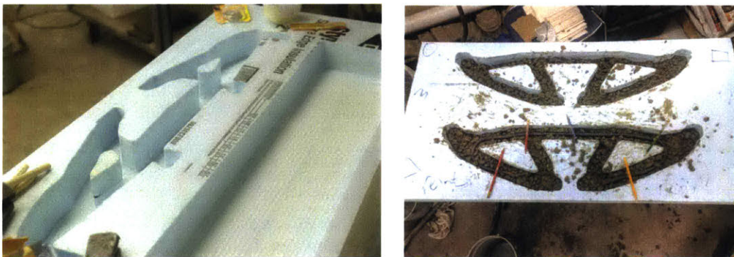
Figure 17: Molds with release agent, and filled with concrete
