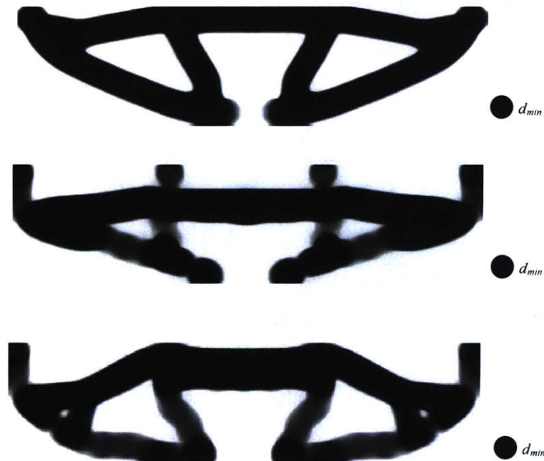
Figure 13: Outputs for Compliance design (top), High Tension design (middle), and Low Tension design (bottom)
