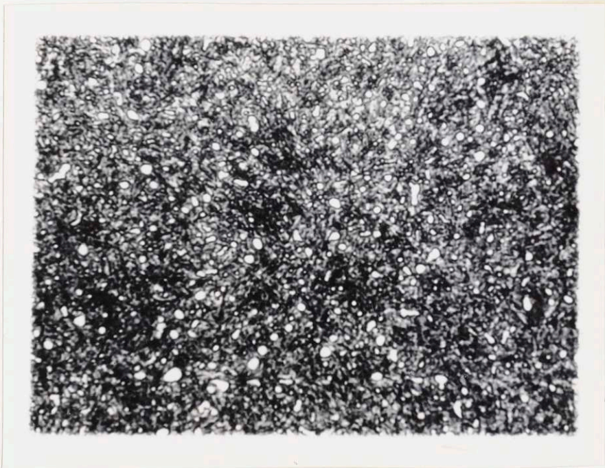
1% C - 5% Cr steel air-cooled from 1700° F., and completely transformed at 600° F.
