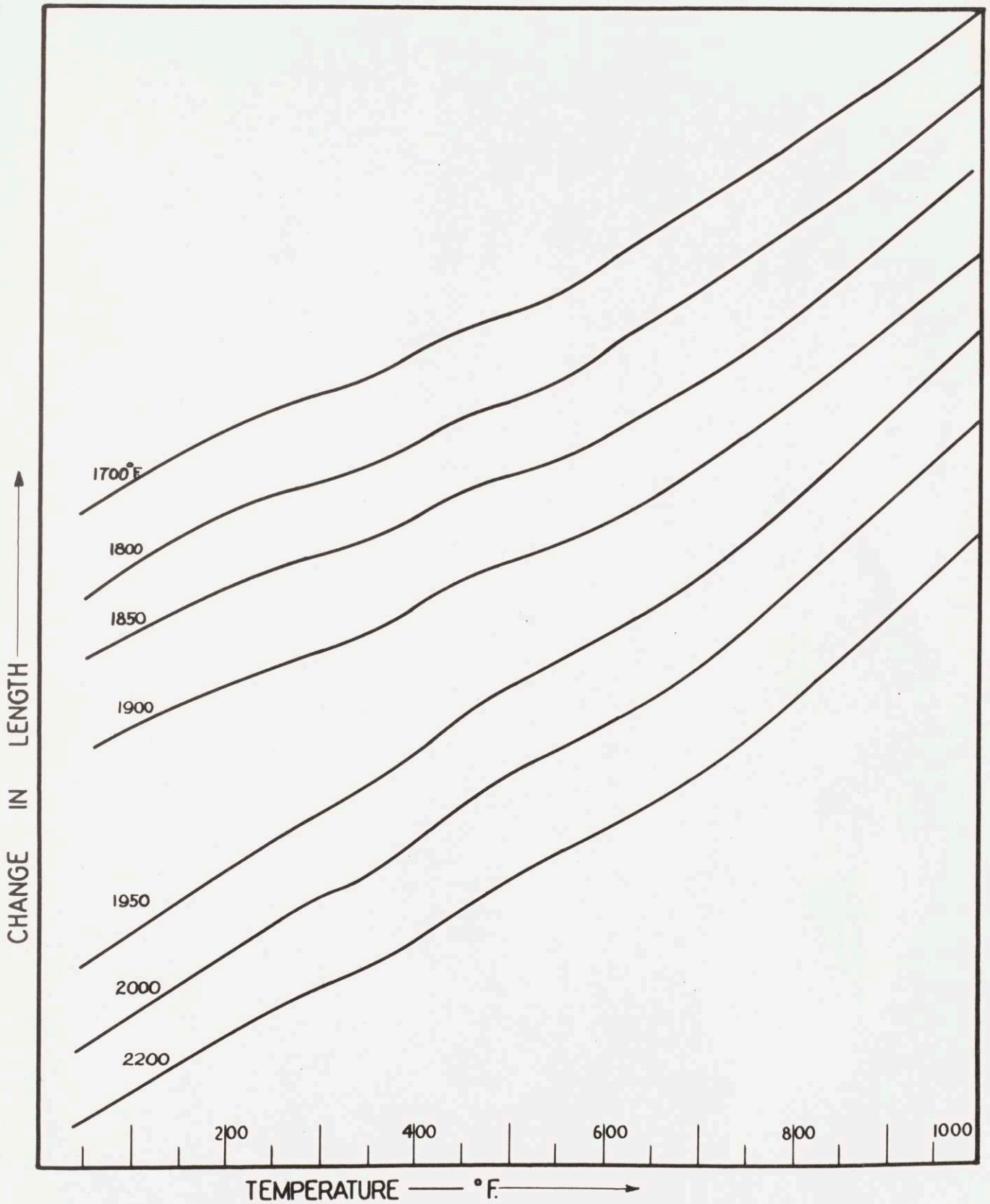
FIGURE 68. HEATING CURVES OF 1% C 5% Cr STEEL OIL QUENCHED FROM TEMPERATURES SHOWN
