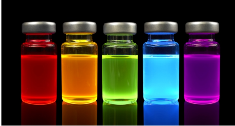
Figure 1.3. Colloidal solutions of semiconductor (CdSe) nanocrystals under ultraviolet illumination exhibiting size-dependent bandgap tunability. Reprinted from ref. 44. Copyright 2016 Nature Publishing Group.
