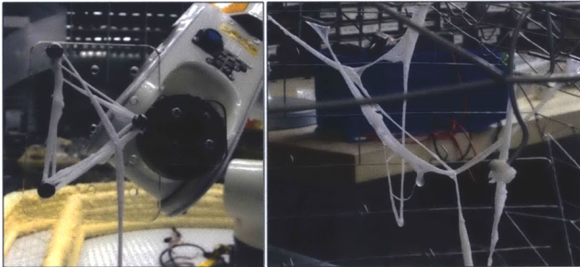
Figure 25. Robotic Arm manipulating the weaving frame that the nylon is being wrapped around. The nylon prepolymer solution is resting on the table below the arm (left). Nylon threads attached to hooks on a steel frame formed by dipping the hooks into a nylon prepolymer solution. (Tsai, Firstenberg, Laucks, Sterman, Lehnert, & Oxman, 2012)
