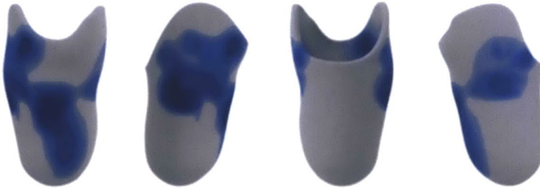
Figure 17. Rendering of the VTS (right limb) with grey representing areas of the socket mapped to hard Objet Digital Materials and blue representing areas of the socket mapped to soft Objet Digital Materials. Softer materials are represented by darker shades of blue. (Left to Right: anterior, lateral, posterior, medial views). Renderings by E.L. Doubrovski.
