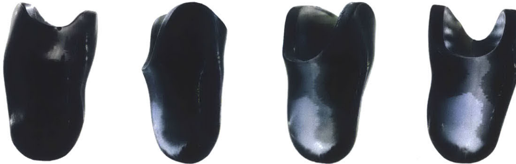
Figure 20. Variable impedance transtibial prosthetic socket bitmap-printed using the Stratasys Objet500 Connex. The darker areas contain higher percentages of the soft rubber-like Tango Black Plus and lighter areas more of the rigid, transparent Vero Clear material. This socket was written on 8832 bitmap files corresponding to 4416 slices and material deposition layers. (Tsai & Oxman, 2013)
