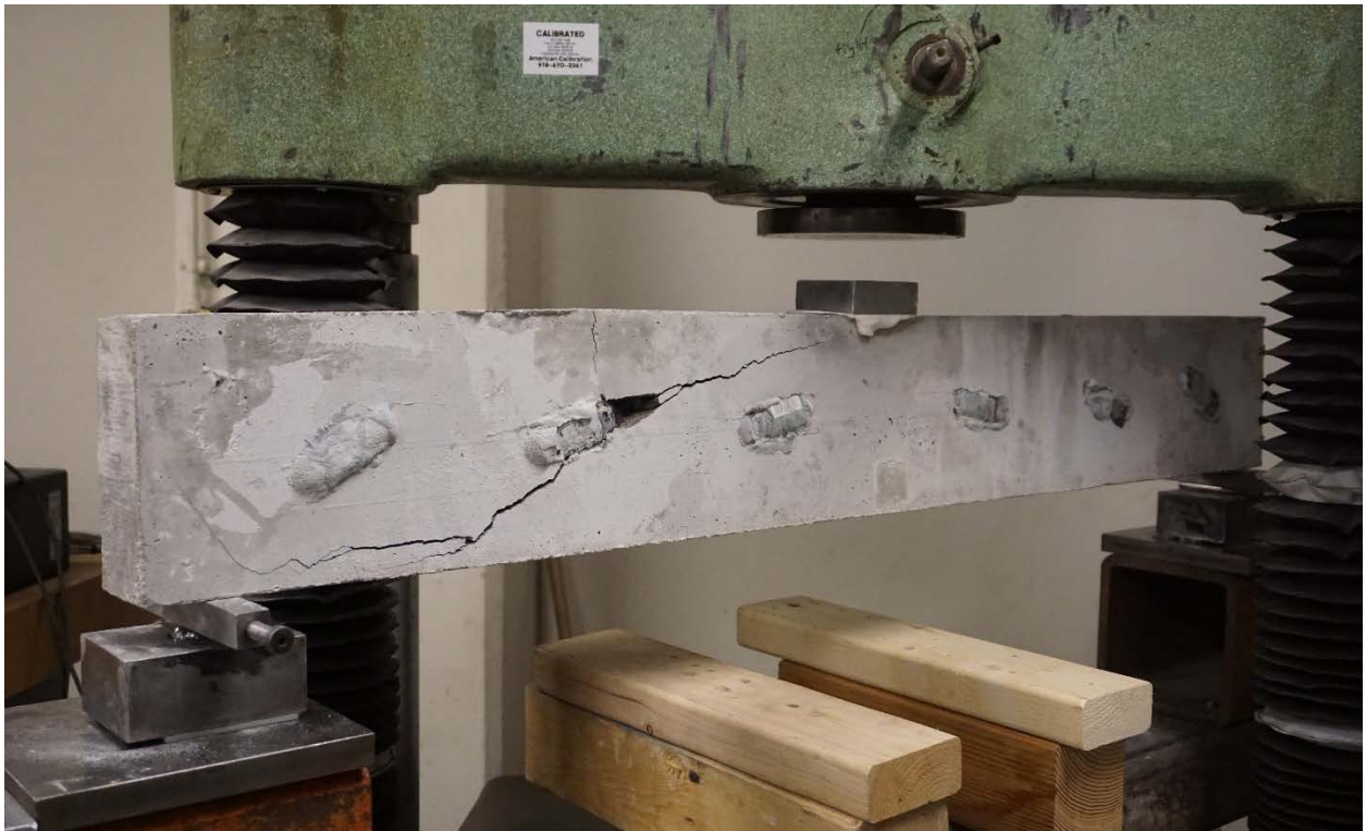
Figure 89 Cavity beam after load testing showing shear failure mode
