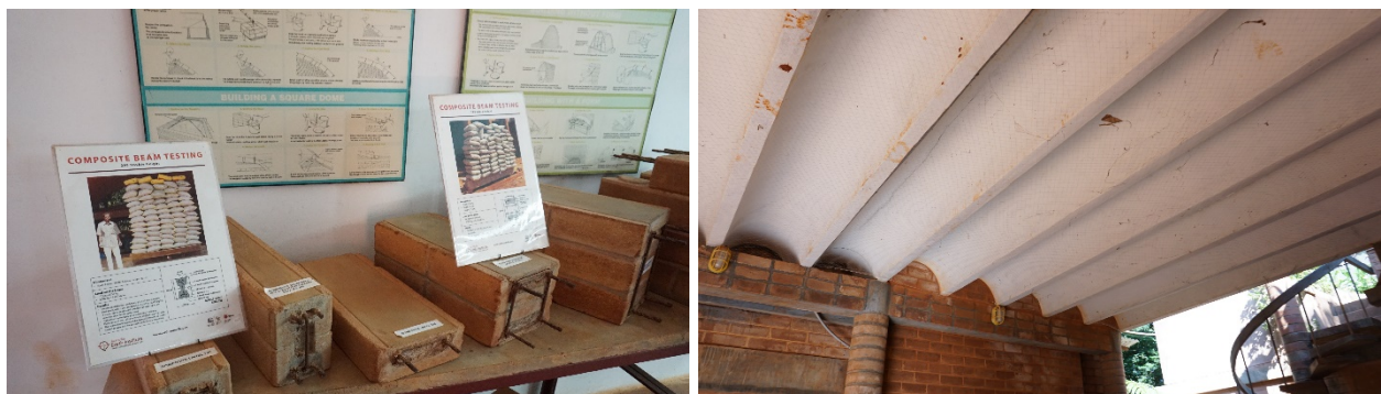
Figure 15 Experiments at AEI in a) hybrid soil-concrete beams and b) ferrocement channels
