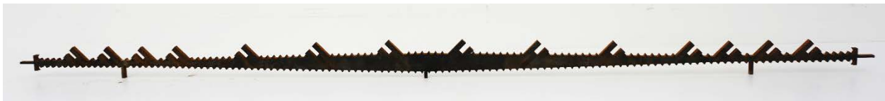
Figure 90 Close up photo of reinforcing cage for CNC bent wire reinforcement
