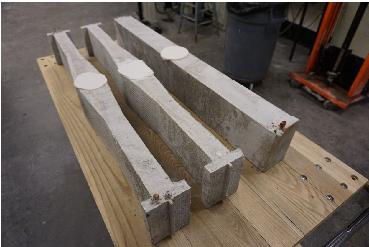
Figure 95 Resultant shaped beams and prismatic control beam
