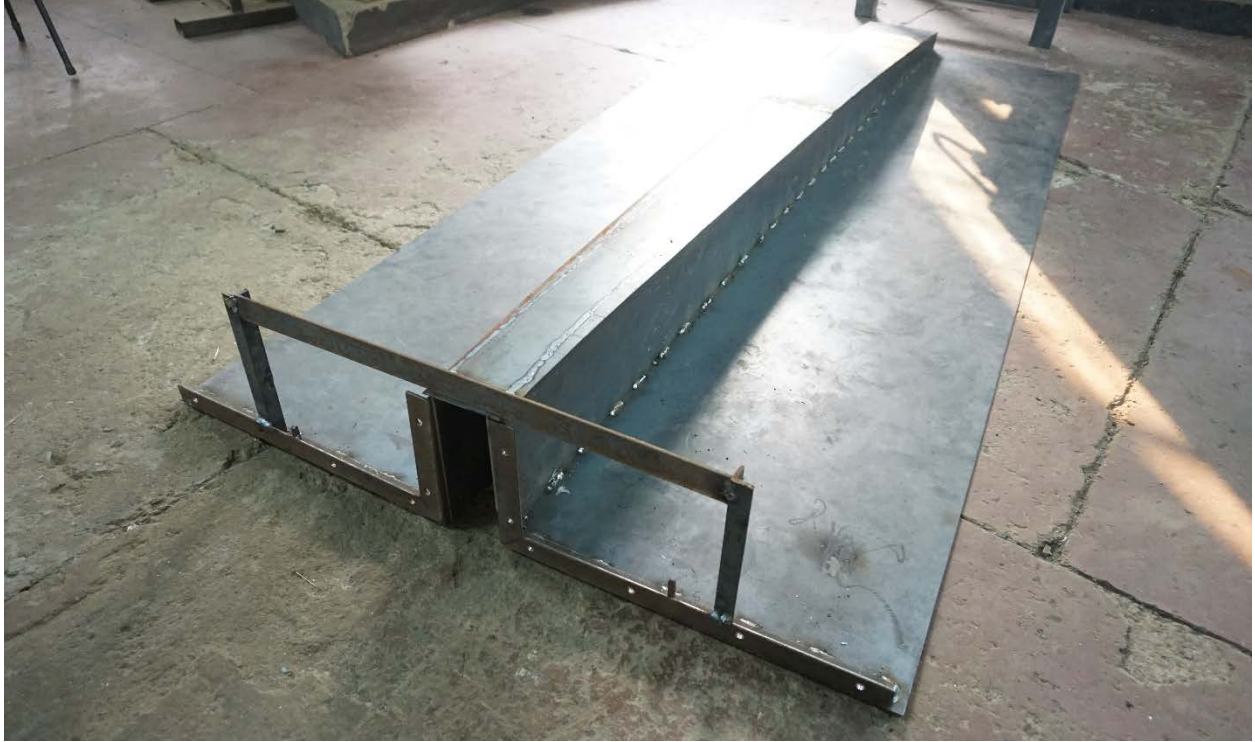
Figure 76 Half of curved sheet metal formwork for full-scale prototype
