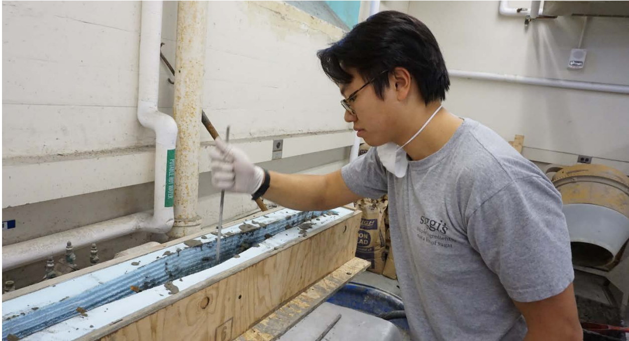
Figure 94 Casting of shaped beam, checking concrete cover on vibrating table
