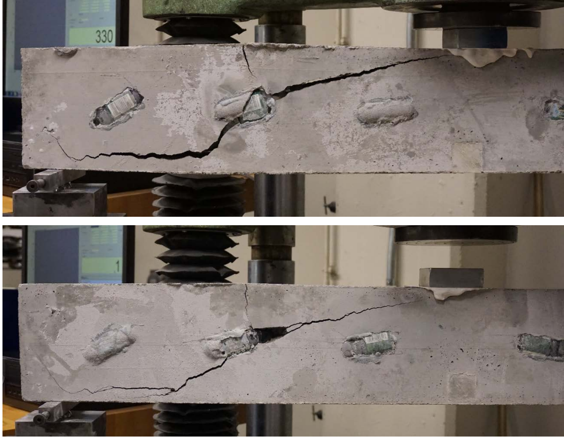
Figure 46 Beams after testing show shear cracks passing from point of loading to supports
