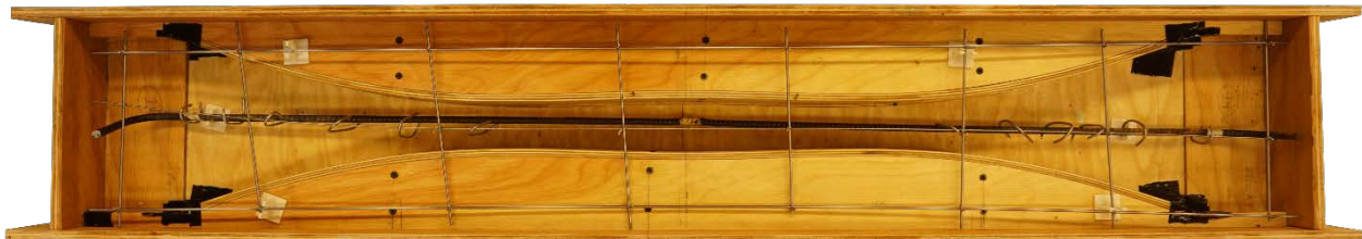
Figure 68 Bent wood form and plywood box for approximated slab fabrication
