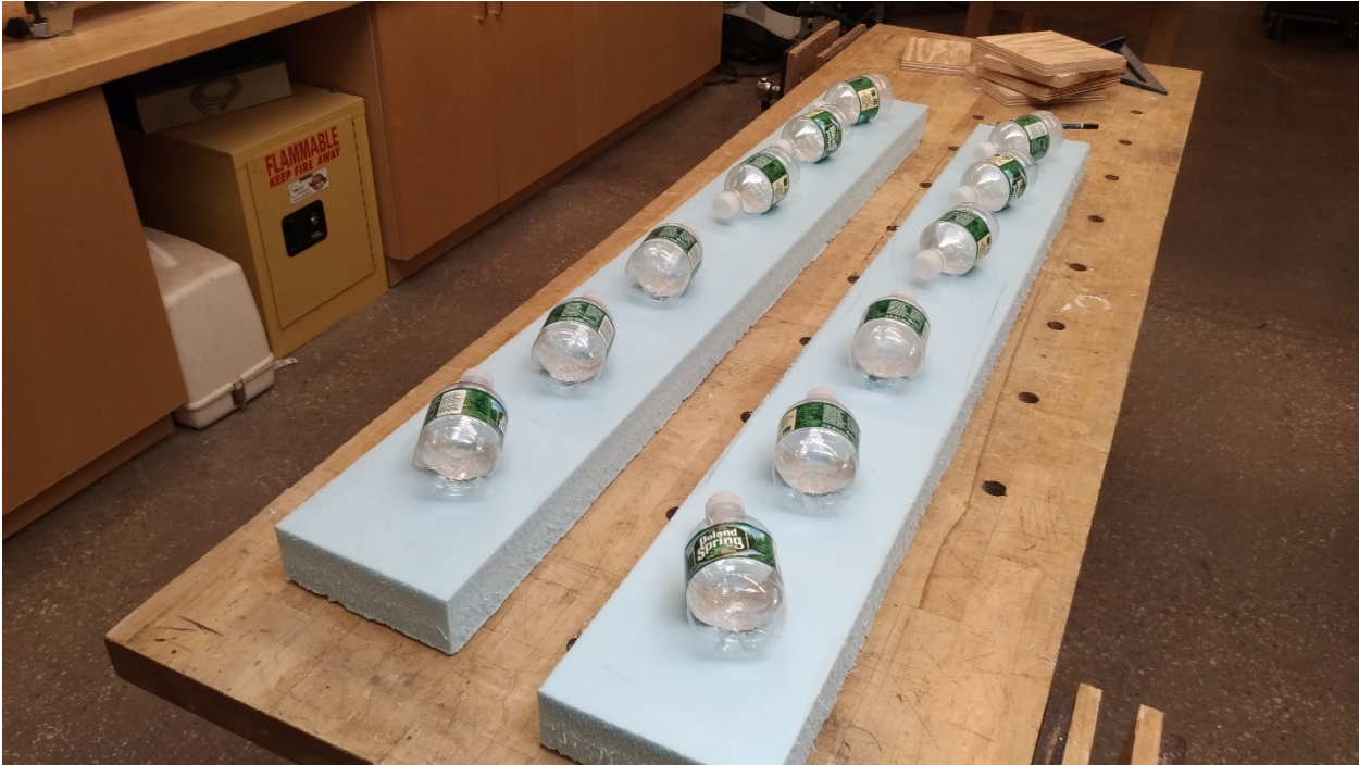
Figure 85 Bottles secured to CNC milled foam formwork
