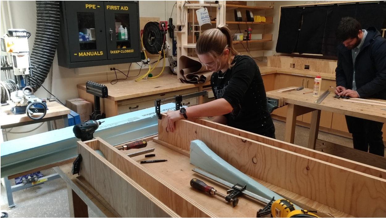
Figure 84 Fabrication of plywood box for cavity beam
