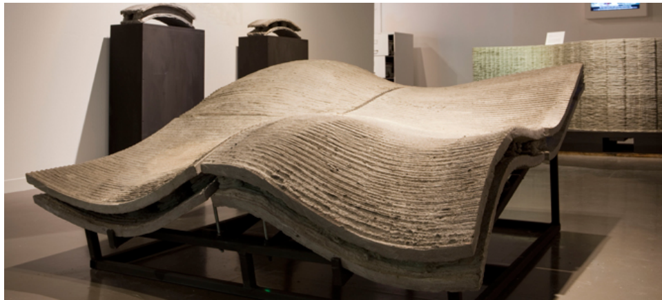
Figure 25 Prototype 3D printed concrete slab, Loughborough University
