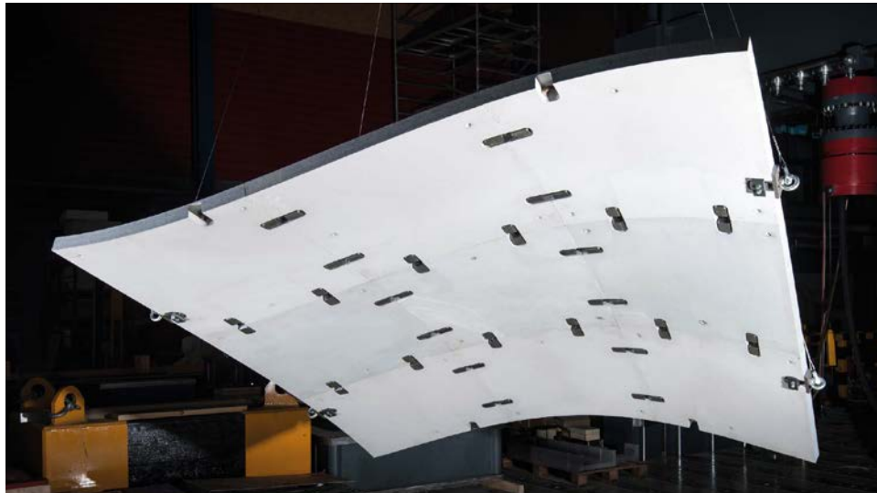
Figure 16 Mock-up of robotically fabricated doubly-curved concrete slab, Graz University of Technology
