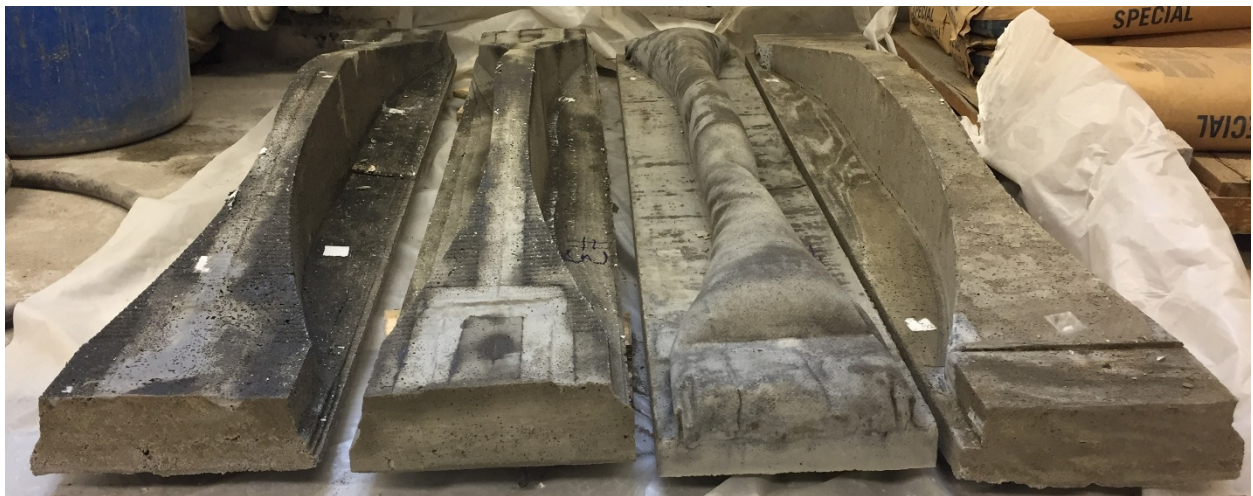
Figure 99 Resultant prototype slabs cast using CNC milled foam, hanging fabric, and bent plywood
