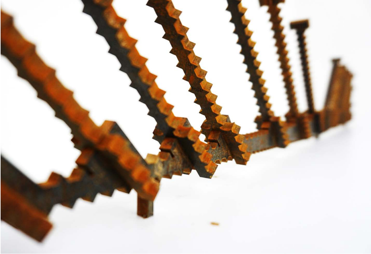
Figure 92 Close up view of CNC waterjet plate reinforcement, connection between transverse and longitudinal steel
