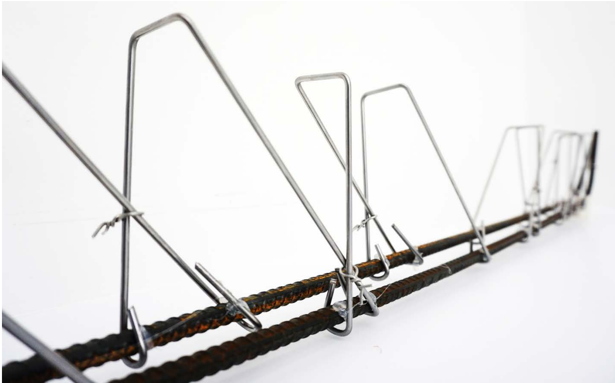
Figure 90 Close up photo of reinforcing cage for CNC bent wire reinforcement
