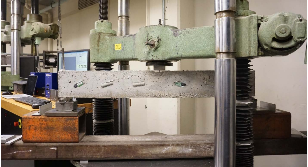
Figure 88 Three-point load test of cavity beam
