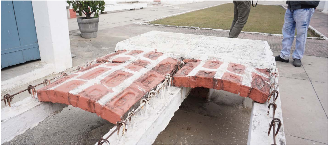
Figure 112 Jack arch and precast beam prototype, Roorkee, courtesy of Central Building Research Institute
