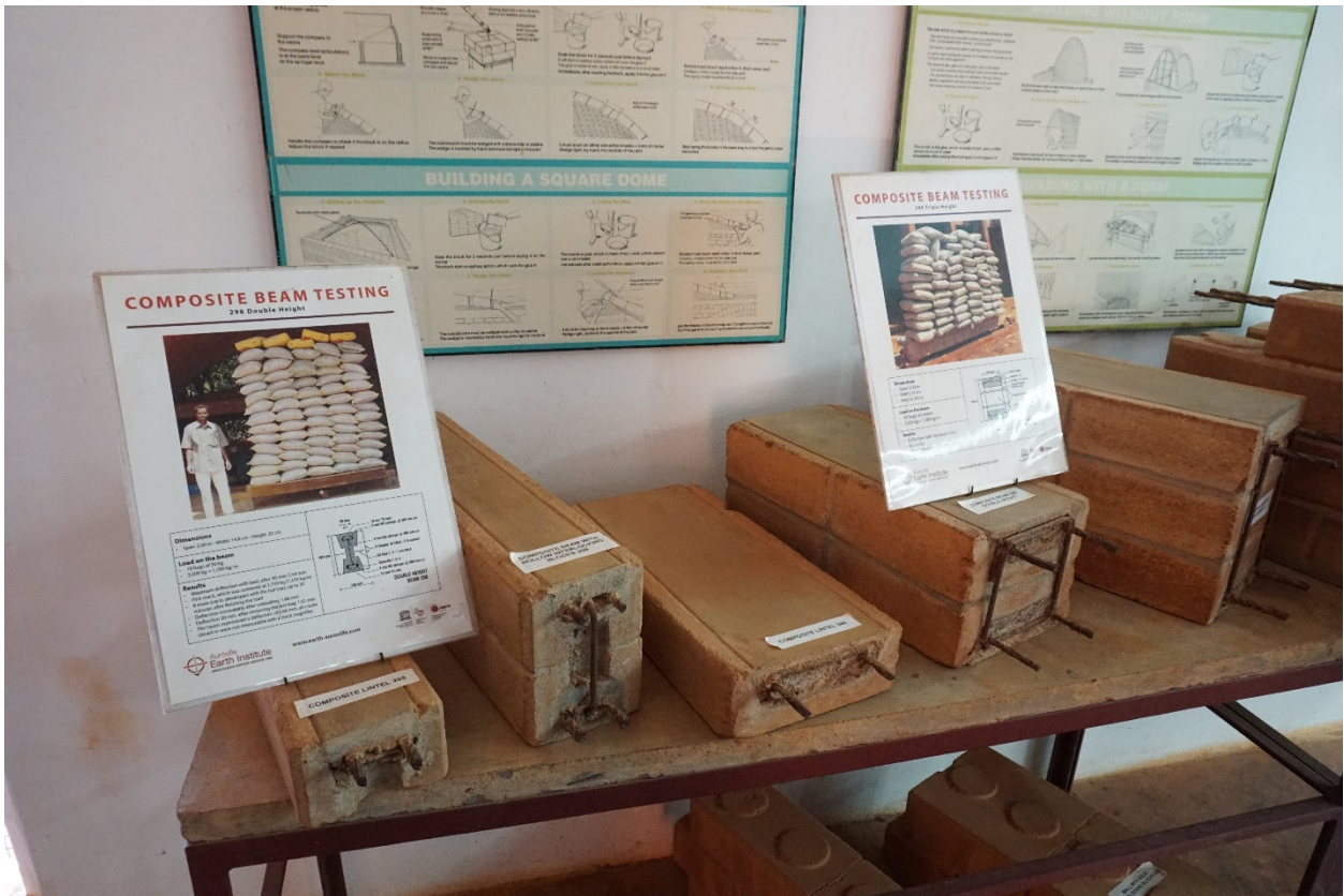
Figure 113 Hybrid soil block and concrete beams, courtesy of Auroville Earth Institute (AEI)
