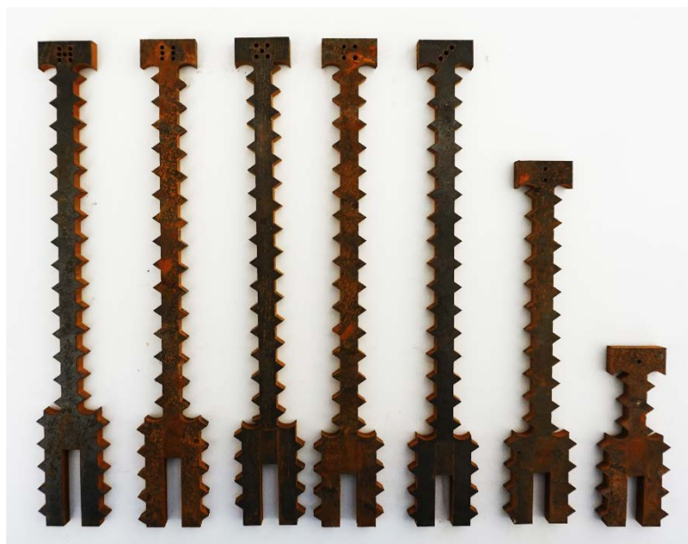
Figure 91 Individual elements of CNC waterjet steel plate reinforcement
