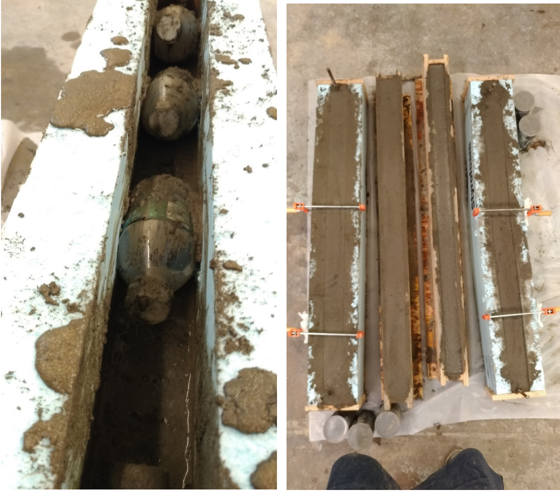
Figure 86 Casting of cavity beams
