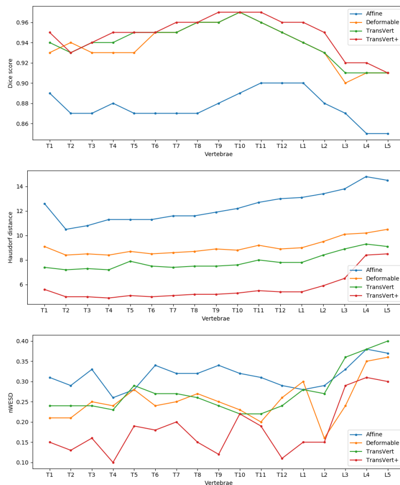
Figure 9. Vertebra-wise comparison of different architectures (Affine, Deformable, TransVert and TransVert+) using Dice scores, Hausdorff and nWESD distances. A higher Dice score indicates better performance. A lower Hausdorff and nWESD distance indicates better performance.
