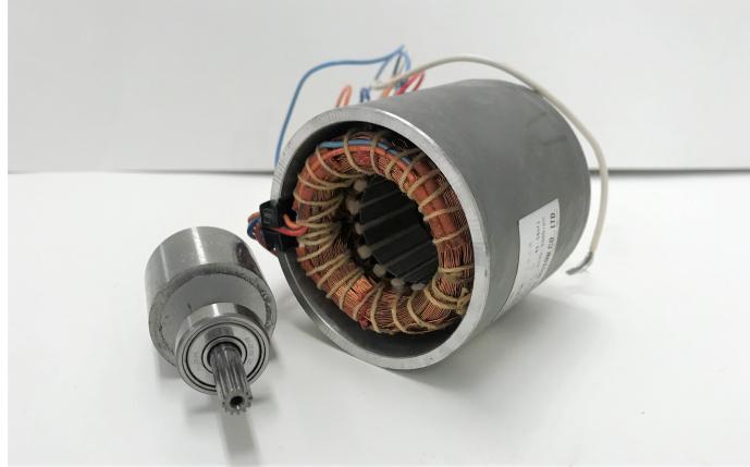
Figure 2-2: Photograph of a legacy off-the-shelf hysteresis motor from Oriental Motor with the rotor taken out. The rotor consists a rotor shaft, an aluminum core, and a ring-shaped hysteresis alloy. Motor was purchased on eBay.
