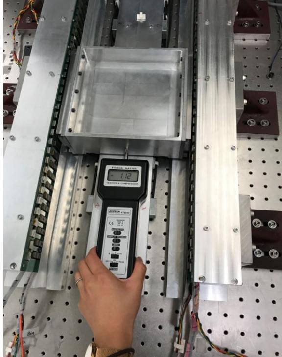
Figure 6-6: Photograph of thrust force measurement process for the linear stage.
