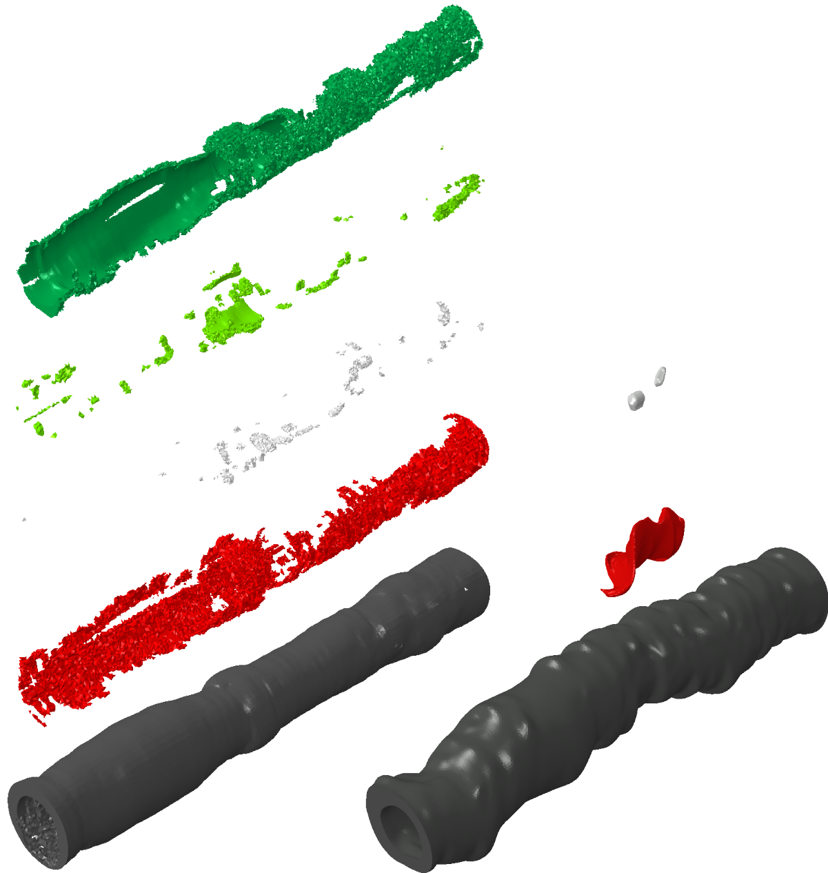
Figure 4.6. The two modeling approaches exhibited tradeoffs in refinement and detail. Whereas generating a monolithic mesh and subsequently assigning material properties ( left ) allowed for substantially more detail to be retained, features were coarse. To the contrary, generating separate geometries for each plaque feature before generating an accommodating cohesive mesh ( right ) was far more laborious and enabled inclusion of fewer features, but included features were much more refined. Note that the two models shown here do not correspond to the same patient, and the latter had not been constructed to include distinct fibrous or mixed tissue—as preliminary (and laborious) work, only a subset of the plaque has been implemented in the model. The resulting differences in plaque representation are reflected in the stress and displacement distributions (Figures 4.4 and 4.5).
