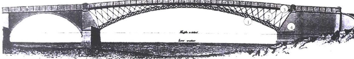
Figure 3.2: Telford's sketch of Bonar Bridge ( Telford, Life of Thomas Telford, Civil Engineer 1838 ), with labels added by the author
