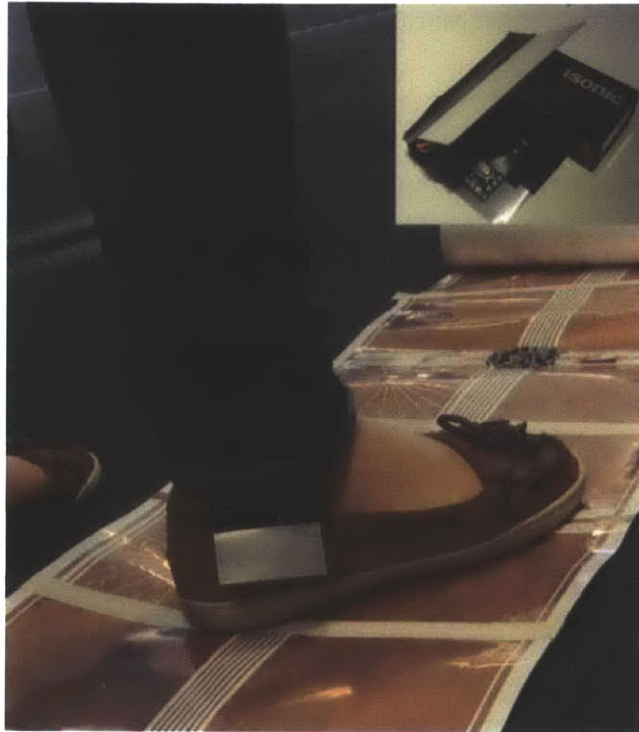
Figure 6.15. Illustration of transmitting/receiving into the floor – from clip on shoe attachment to the sensor floor tiles.
