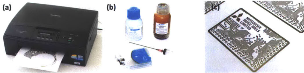
Figure 3.2 Conductive Inkjet printing with off-the-shelf printing and conductive silver particle ink. (a) An example inkjet printer with silver nano particle filled ink cartridges. (b) Silver nano ink and replacement ink cartridges. (c) Example printout from Mitsubishi paper mills limited.
