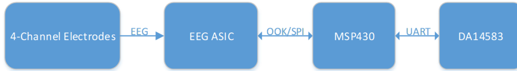
Figure 3-1: Wearable System Block Diagram showing the main functional components of the patch EEG.
