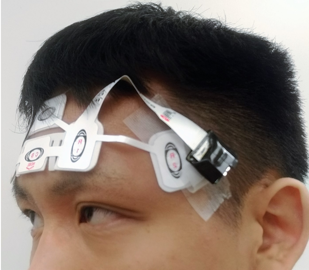
Figure 3-7: Wearable System Testing. Electronics package in black is adhered on the temple.
