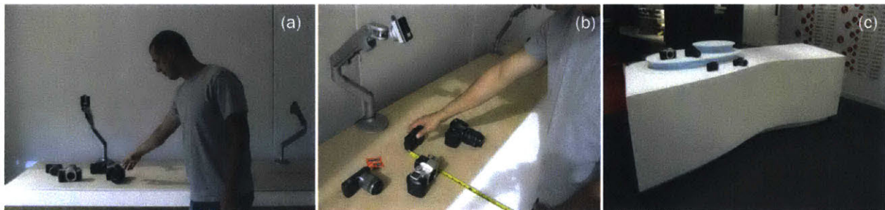
Figure 5-14 Designing the APC interaction space: (a) measuring users' reach (b) measuring product distribution and projection real-estate (c) the APC foam-core mock up
