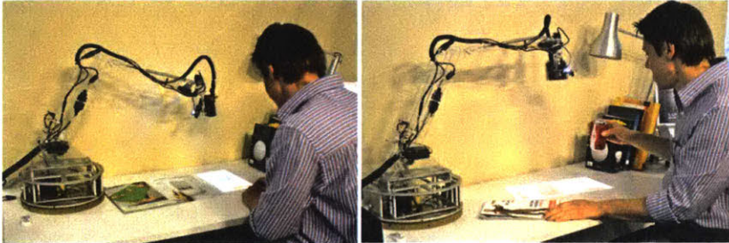
Figure 5-13 Early object augmentation explorations using LuminAR Optimus. The lamp detects objects like a magazine or a can of soda using simple fiducial markers, once detected the objects are augmented with relevant web content.
