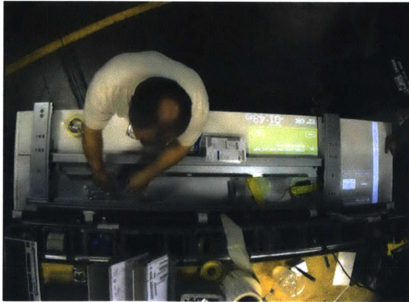
Figure 7-1 MARS enabled AR assembly process in Steelcase Kentwood West Factory
