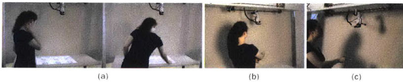
Figure 3-41 LuminAR Spotlight interaction techniques include: (a) projected multitouch, (b) hand tracking and, (c) tracking fiducial markers
