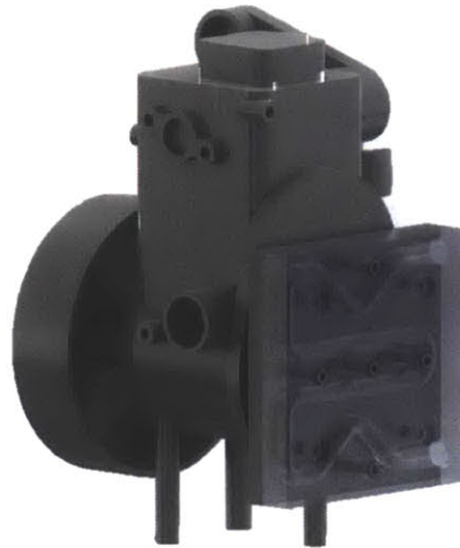
Figure 8.4: Model of GXH50 Engine with Cooling Block Attached
