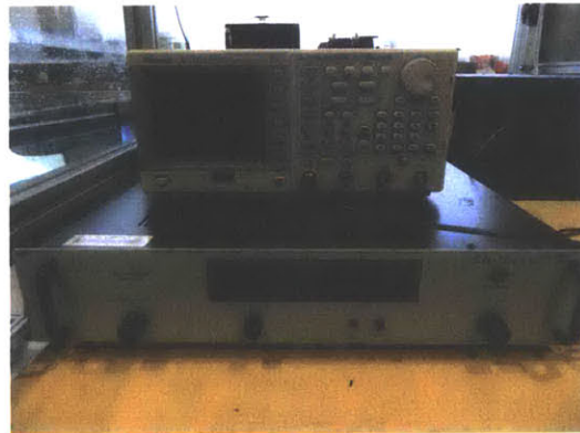
(c) Power amplification for the mini shaker was provided by a Brüel and Kjaer Type 2718 power amplifier.
