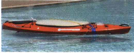
Figure 2-13: An unmanned kayak, used in radio control mode, was used as a platform for testing multiple arrays of experimental pressure sensors.
