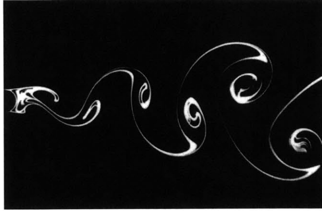
Figure 7-1: The periodic shedding of vortices behind a bluff body in a flow field is known as the Kármán vortex street, and has a shedding frequency related to the flow velocity and body size by the Strouhal number (adopted from [29]).
