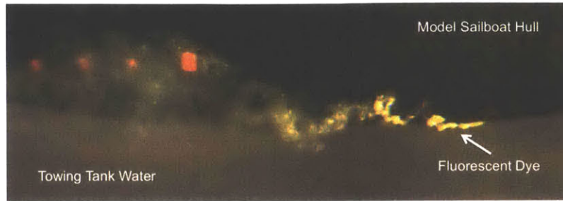
Figure 2-5: When towed at an angle of attack, even well streamlined hull shapes, such as a model sailboat hull, present a bluff cross section to the incoming flow field. This drastic change in cross section results in the shedding of strong helical vortices from the hull's keel line. These helical vortices were visualized in the MIT Towing Tank by injecting fluorescent dye into the flow field at the keel line, near the bow of a sailboat hull. The dye could be clearly seen curling into a helical vortex that grew in diameter towards the stern of the model, and began to break apart due to the effects of viscosity.
