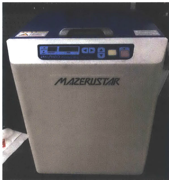
(c) During fabrication, CB particles were mixed into Part A of the Soma Foama silicone foam using a Mazerustar high speed mixer to ensure even distribution of particles throughout the composite.
