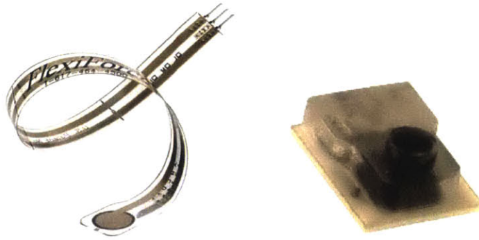
(a) Flexiforce conductive ink (b) The model 1620 disposable sensors from Tekscan showed medical pressure sensor from Measurement Technologies had great form factor and flexibility, but lacked the sensitivity required for near-body flow sensing. a dielectric gel barrier to protect the piezoresistive sensor die from contact with fluid, but lacked the form factor for surface-mount applications.
