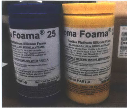
(a) Closed-cell CBPDMS foam was produced using Soma Foama, a two part platinum silicone foam from Smooth-On.
