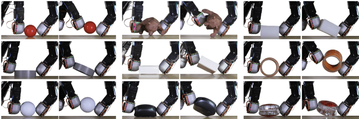
Figure 6-1: Sample begin and end state of each object during the rolling phase of the experiment in the controlled rolling task.
