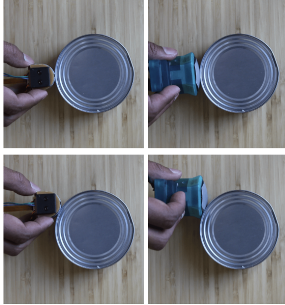
Figure 3-2: Human demonstration illustrating contacts made on different parts of a cylinder using the finger’s transverse plane. (a) the contact areas made with a curved finger,(b) the contact areas made with a flat finger. The round finger keeps a consistent contact area at each contact point unlike the flat finger.
