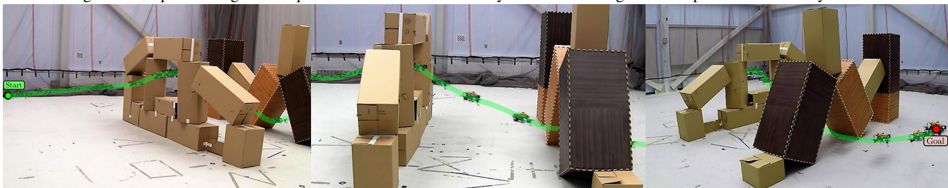
Fig. 25: Composite image of Experiment 2. The UAV must fly from start ● to goal ●. Snapshots shown every 330 ms.
