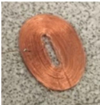
Figure 6-3: A coil of wire with each ends attached to a cylinder for fixture.
