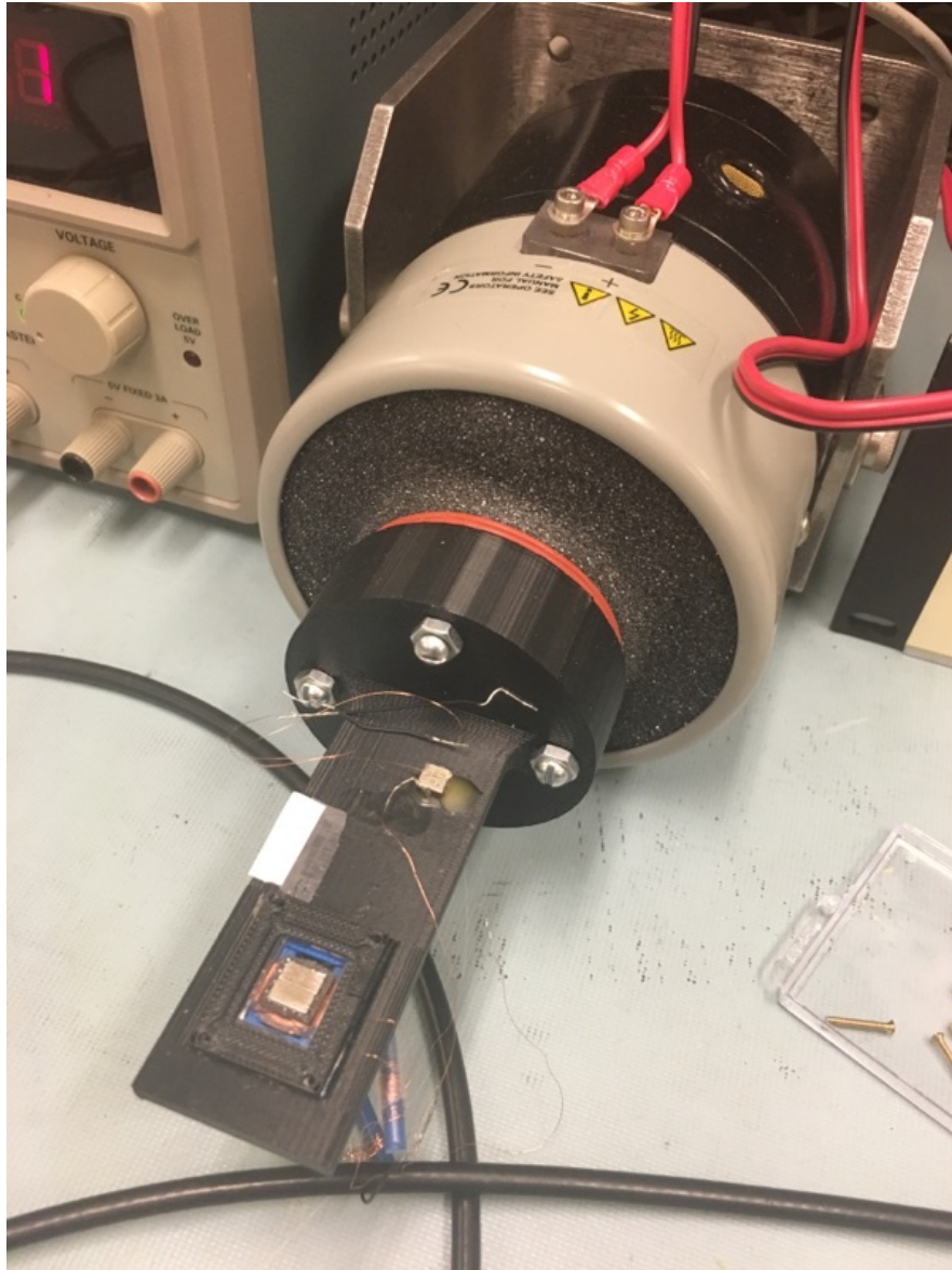
Figure 6-7: Fully assembled harvester on a vibrating platform that is connected to the mechanical vibration machine.
