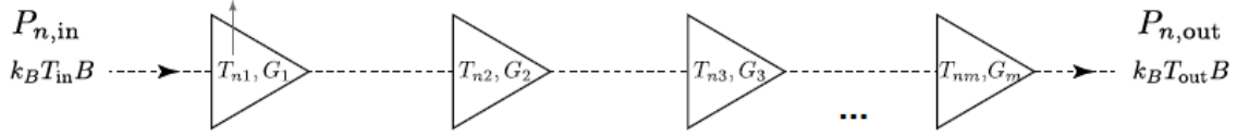
Figure 2-1: Simplified measurement chain featuring multiple amplifiers, adapted from [1]. The Friis equation indicates that the noise temperature of the first amplifier in the chain dominates the overall output noise.
