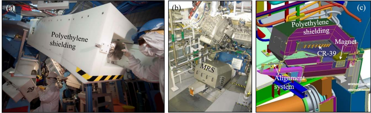
FIG. 5.16. (a) The OMEGA-MRS fully enclosed by polyethylene shielding. (b) The NIF-MRS fully enclosed by polyethylene shielding. (c) Cut-out view of the NIF-MRS illustrating the spectrometer inside the shielding. The picture in (c) is taken from the paper by Frenje et al. [5.54].
