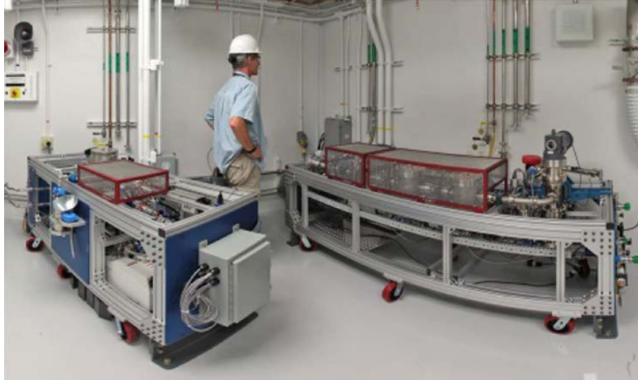
FIG. 8.1. The RAGS hardware at the NIF. Directly after a shot, the gaseous products inside the target chamber are pumped out and into RAGS, where unwanted species are filtered out from the gas (this happens in the right cart shown in the figure). The noble gases are subsequently frozen and analyzed to quantify the number of nuclear reactions that occurred in an implosion. This happens in the left cart shown in the figure. This picture is taken from the paper by Shaughnessy et al. [8.1].
