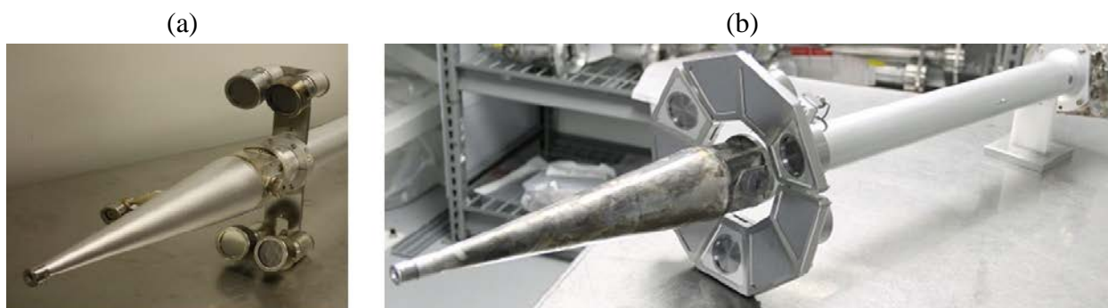
FIG. 8.2. (a) Pictures of the SRC systems. (a) The SRC with a 2-inch diameter disc of either tantalum, vanadium or carbon. Up to four SRC systems can be fielded on one DIM. This picture is taken from the paper by Shaughnessy et al. [8.3]. (b) The Vast Area Detector for Experimental Radiochemistry (VADER) system for solid radiochemistry collection.
