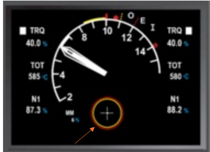
Figure 31: Example Cyclic / Aircraft center position for Pilot Flight Display (“UH-72A Aircrew Training Manual” 2020)
