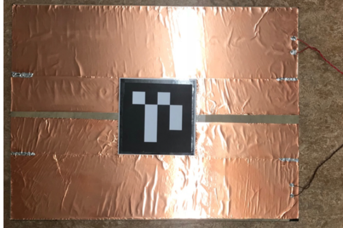
Figure 5-6: The wired contact charging platform with conductive surface and an ArUco Marker.
