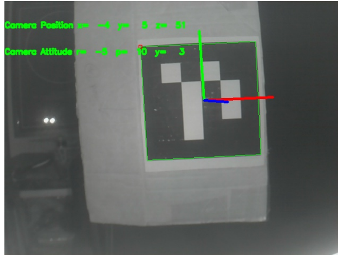
Figure 4-6: ArUco marker detected by the night vision camera with marker coordinate system axis drawn in the dark environment [9]. The position and the attitude of the camera in respect to the marker are shown in the text on the top left side.
