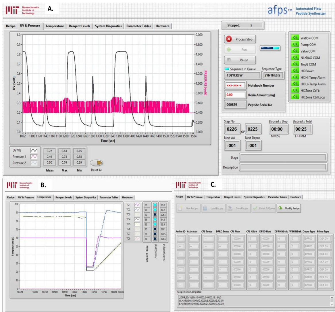
Figure 2.5: General Labview VI for the AFPS
