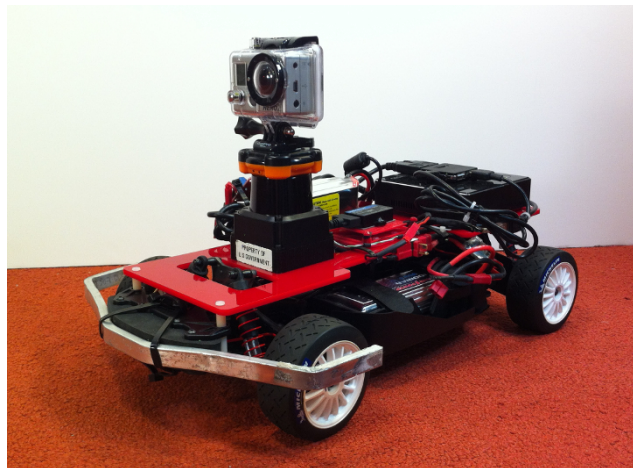
Fig. 9: 1:8 scale RC car used in experiments, with Hokuyo laser range-finder, Microstrain IMU and computer.
