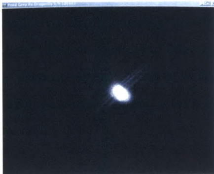
Figure 4-4: Image of the laser dot used for the centroid calculation time measurements
