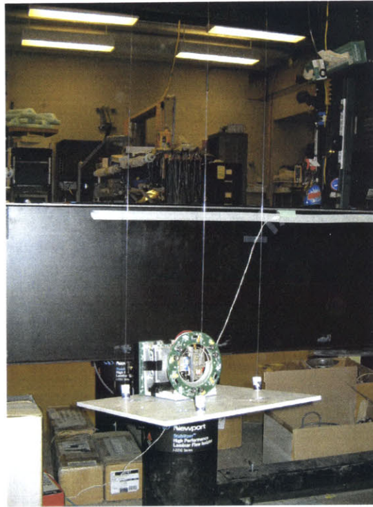
Figure 4-10: Estimating the moment of inertia of the Precision Pointing Optical Payload using a hanging pendulum
