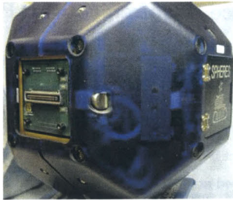
Figure 2-4: SPHERES Expansion Port
