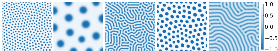
Figure 5-2: Examples of Di-BCP melt microphase separation simulated using the OK model for various choices of the model parameters (m, \epsilon, \sigma) . The two phases are indicated numerically as -1 and +1 .
