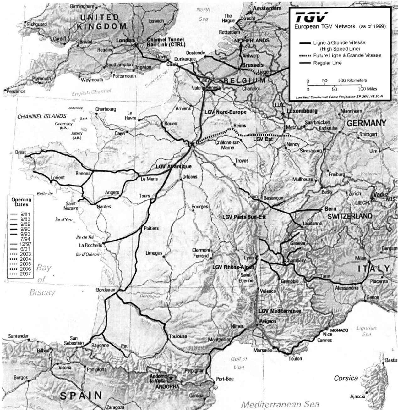
Figure 2.5 TGV Dedicated Line Network Expansion
