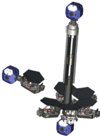
Figure 1-7: Proposed project for robotic assembly of a space telescope [25]
