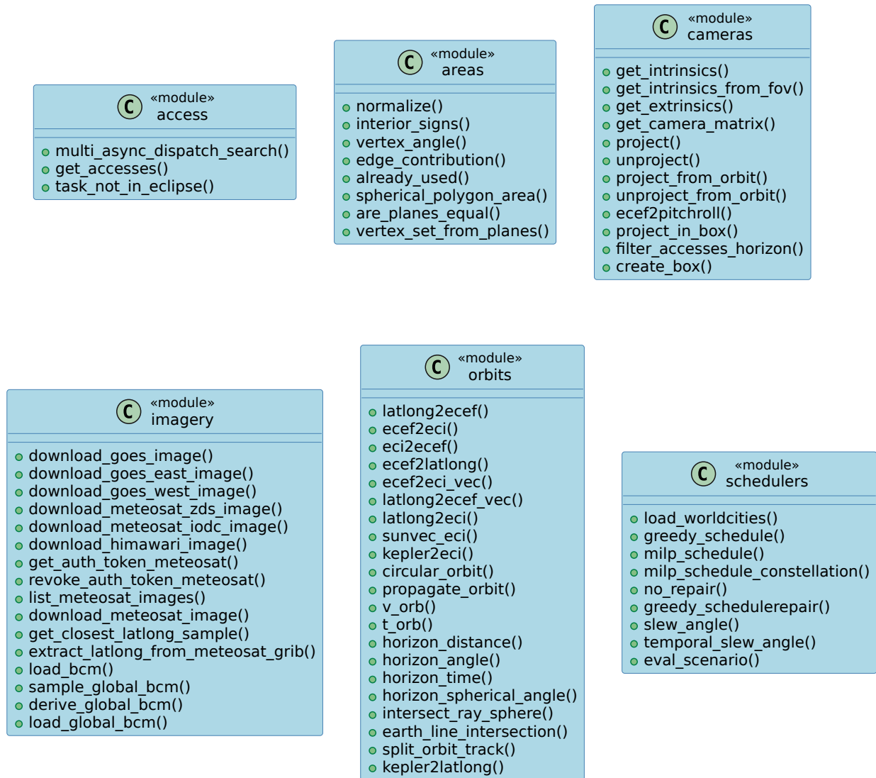
Figure 6.8: Diagram of dynamic_tasker.py software package, showing core modules and functions enclosed within each module.
