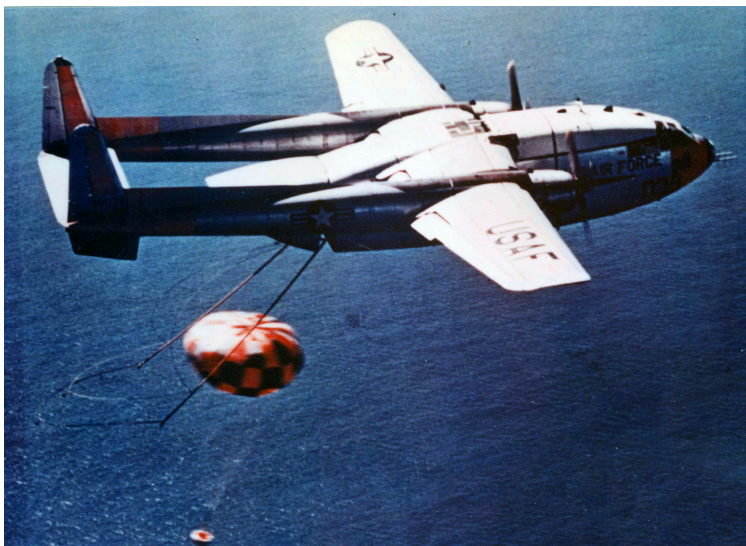
Figure 1.2: Recovery of a Corona film canister in mid-air from a Fairchild C-119 Flying Boxcar aircraft (1960) [10].
